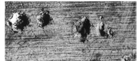
Fusion craters in a bearing race from Scanning Electron Microscope image
