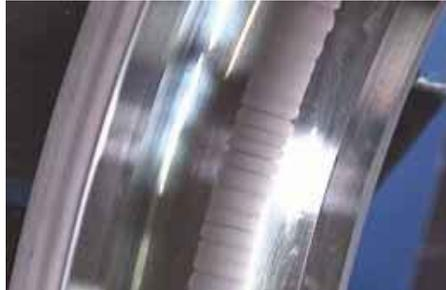
Fluting or washboard in raceway
