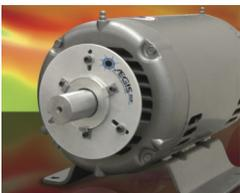
This is a Nema/IEC Mounting Adaptor to facilitate installation of the device on AC motors with shaft shoulders, slingers, bearing caps, or end-bell protrusions. Designed for use on any NEMA or IEC motor frame, the adaptor consists of a mounting plate to support the SGR and standoffs to provide clearance for bearing housings or slingers. Available for Nema 56 thru 449T frames and 80 frame thru 355M frame IEC
