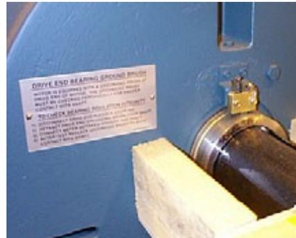
A metal brush contacting the motor shaft is a more practical and economical way to provide a low-impedance path to ground, especially for larger NEMA-frame motors. However, these brushes pose several problems of their own:
