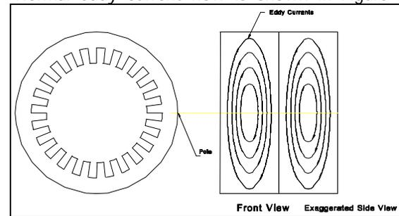
Figure 2 - Normal Eddy Current Flow
