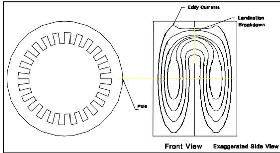
Figure 3 - Interlaminar Eddy Current Flow
