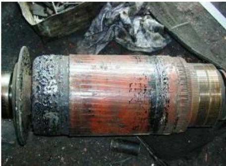
Here we see the Armature with its winding and the Commutator, where all the Armature wires connect to. Brushes ride on the Commutator surface and they provide the means of feeding the necessary Armature current into the Armature itself.
