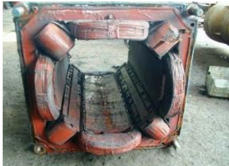
In the end view of the disassembled motor you see 4 narrow windings, Interpoles, and 4 wide windings, Shunt fields.
