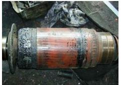
Here we see the Armature with its winding and the Commutator, where all the Armature wires connect to. Brushes ride on the Commutator surface and they provide the means of feeding the necessary Armature current into the Armature itself.
