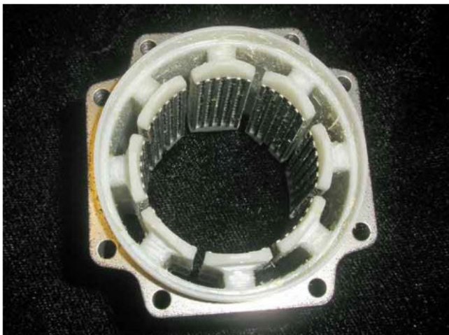
Stator with All of the Wire Removed.
