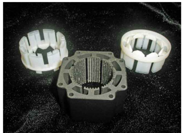
Insulator Halves Slide in from Both Sides. Coil Wiring Holds them Together.
