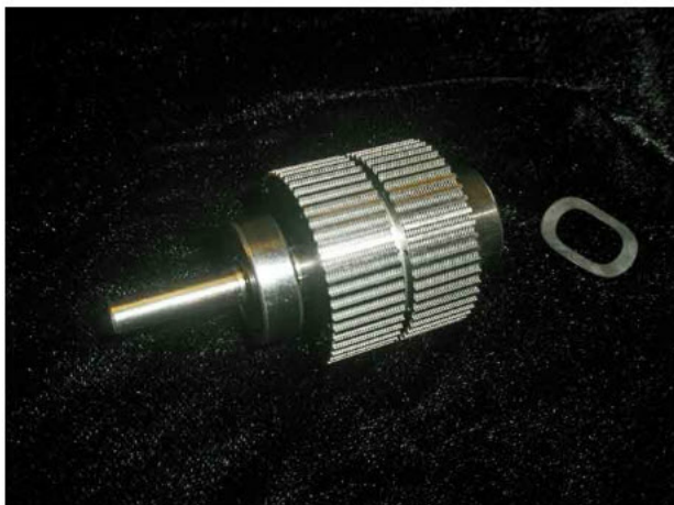
Rotor Removed. Note Bearings Pressed on Both Sides. The Rotor is Really a Stack of Around 60 Magnetic Disks
