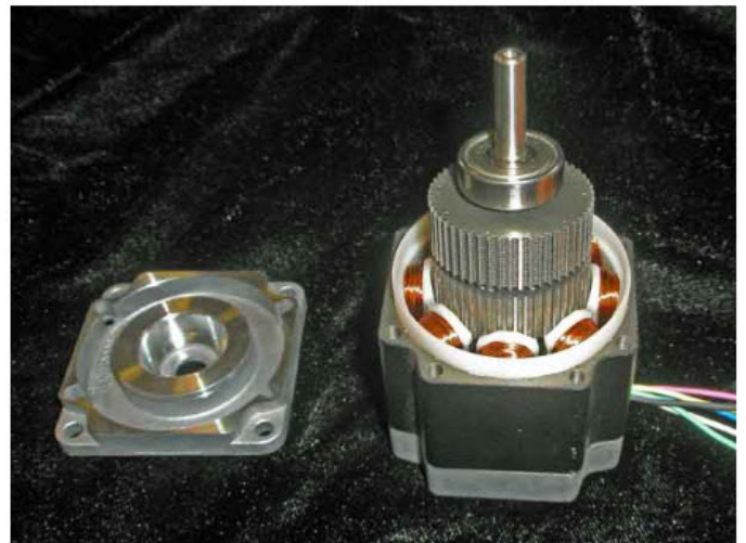
The Rotor Slides Right Out
