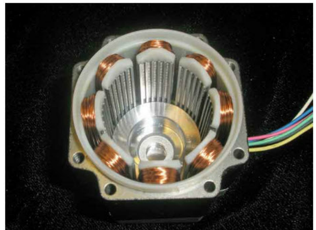
Stator with Windings. You Can See the Race Where the Bottom Bearing Rests.
