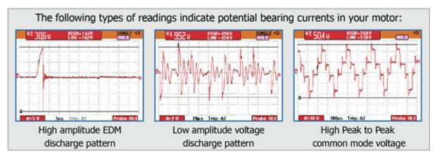
It should be mentioned that not all motors driven by a VFD suffer from electrical erosion, although the potential risk is always present.
