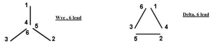
Now when a winding is designed each phase winding is rated for a certain voltage. If you put too much voltage across the winding the winding will be too strong and will overheat. If you put too little voltage across the winding it will be too weak and not develop the torque you want.
