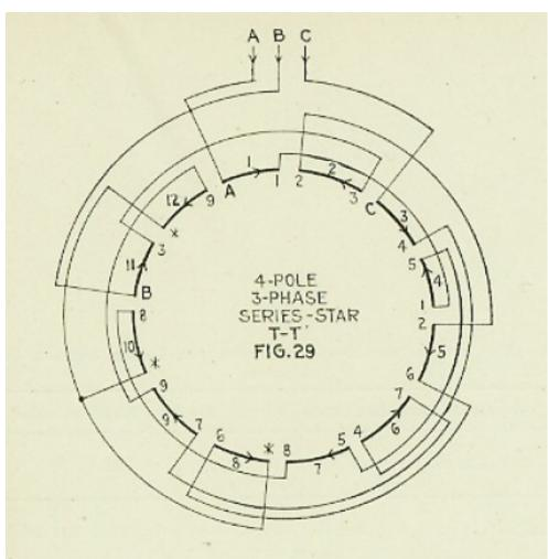
This picture shows a connection diagram for a simple 4 pole (1800 rpm sync. speed), 12 group, 3 phase motor, with a 1 Wye (series star) connection.
