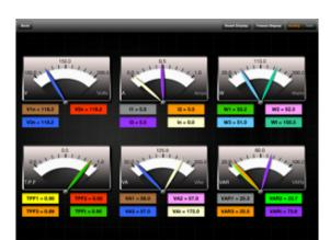
Analog or Digital real-time meters - you get both! Each meter group can be expanded to show individual phases.
