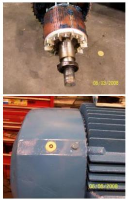
Shown on the left is the plastic plug covering the grease fitting, on the right is our mod to show the grease fitting. The original grease fitting was about 2" below the fan cover plug, we extended it out to be flush.
