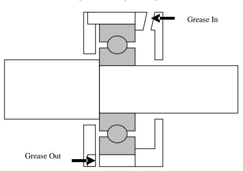
Figure 1: Bearing Greasing
