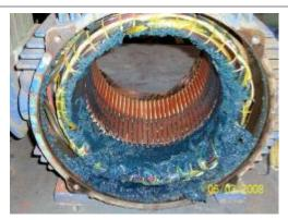
Above and below we see what happened at the motor shaft end of the motor. Much too much grease here. Led to motor winding shorting out.
