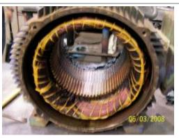
Here we see what happened at the opposite end of the motor. No grease here on winding, same with rotor
