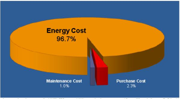
(The data above was based on a test of a 11kW IE3 motor,4,000 operating hours per year,15 year life cycle. Source: EuP lot 11,2008)
