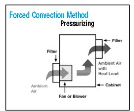
The Pressurizing Forced Convection Method( on right above) is preferred in that only air filtered by the fan flows into the switch cabinet.
