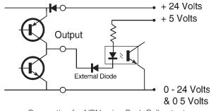
Connection for NPN using Push Pull output NOTE: Common 0 Volt Supply
