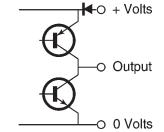
Connection for normal Push Pull output
