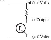
PNP or current source: Has a 40mA switching action between the + Volt supply and the output. Pull down resistors are fitted between the output and the 0 Volt power supply line.
