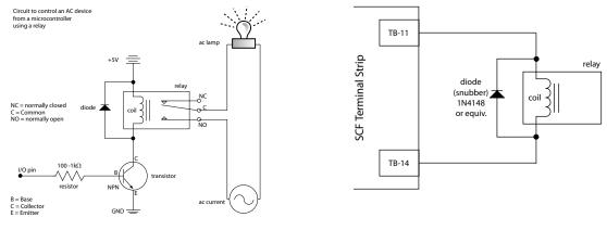
Figure 2a: Relay Control Circuit (Generic)
