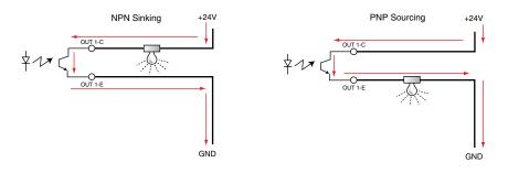
Figure 1: Current Sinking (NPN) and Current Sourcing (PNP)
