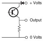
Line Driver: Uses a push pull line driver output circuit which provides a 5 to 15 Volt 40mA output signal capable of driving cable runs up to 100 metres.
