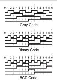
The main consideration is that standard Absolute encoders only provide this feature for one shaft revolution. Therefore their use is restricted to synchronising machinery based on a 360° cycle. If more turns are required it is necessary to use some form of mechanical reduction, or select one of our Multi-Turn Absolute encoders. This type has an internal mechanical arrangement that drives multiple absolute code disks.
