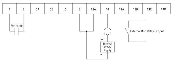
Figure 4: Wiring the Open-Collector Output of the MC Series Drive
