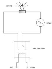
Figure 3: Typical Relay Circuit
