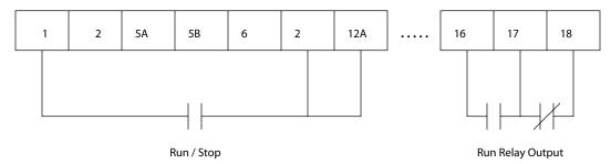
Figure 5: Wiring the Form-C Relay Output of the MC Series Drive
