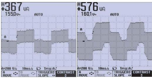
Figure 3C. Normal PWM waveform.
