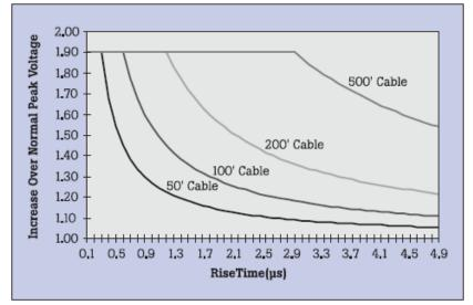
Figure 3B. Impact of rise time and cable length on magnitude of reflected voltages.
