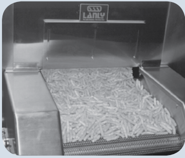
MTS Sprockets and mesh convey cheese puffs through this Lanly oven highly effectively.
