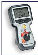
With hand-cranked Megger instruments, it's a lot easier for you to run the test for only 60 seconds, taking your first reading at 30 seconds. If you have a line-operated or a new type electronic Megger instrument (like Megger MIT 420), you'll get best results by running the test 10 minutes, taking readings at 1 and at 10 minutes, to get the polarization index.
