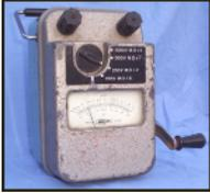
When testing the Insulation Resistance of an electric motor we usually use a Megger. This tester can perform a single test for approx. 60 secs, called a Short-Time or Spot-Reading Test, giving a reading of so many ohms to ground. Insulation resistance should be approximately one megohm for each 1,000 volts of operating voltage, with a minimum value of one megohm.
