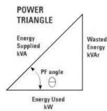
Apparent power is the numerical product of volts and amps.
