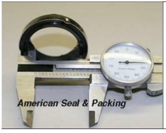
Measure the Seal Head I.D. Add approximately .016" to account for the squeeze the bellows must have to seal the shaft.
