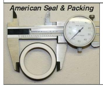
Measure the O.D. of the seat or measure the Bore the seat will press into. If measuring the Outside Dimension of the seat (as pictured) SUBTRACT approximately .016" to account for the rubber squeeze required for the interference fit of the seat.
