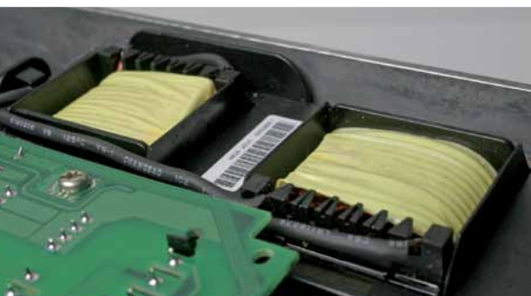
DC coils reduce harmonic noise and protect the drive.
